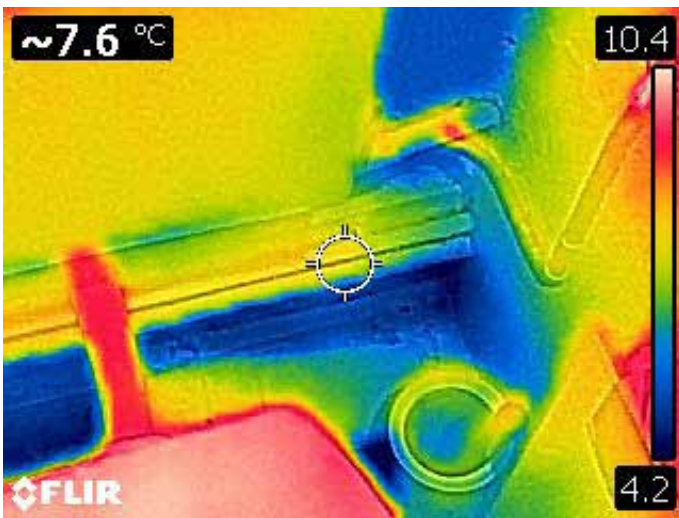
Lots of draughts and leaks are caused by poorly-sealed building services - such as around waste pipes from bathrooms. It's a relatively simple job to just seal these better.
