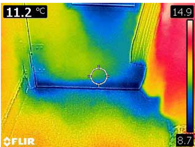
Heat-loss at flat entrance door threshold. A draught-excluder makes some difference here - but full draught-stripping would also help.
